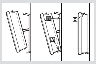
NOTE: If you need to remove the thermostat, follow step 1 in section 1, then use a straight screwdriver to unhook it from the top of the mounting plate.
