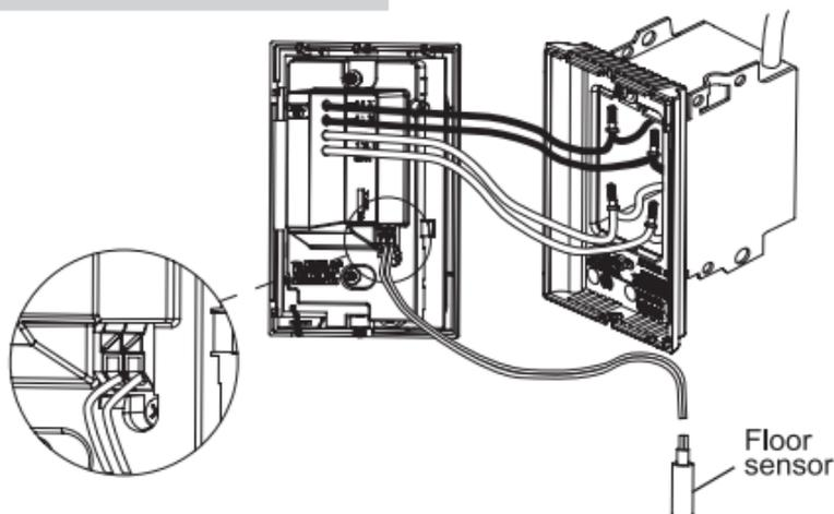
6. Reinstall the front part of the thermostat on the mounting base and tighten the screw at the bottom of the unit.
