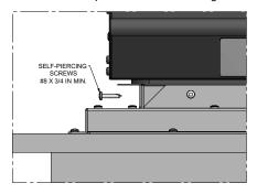
N.B. If the four sides of the furnace are accessible, it is necessary to install two screws per side. If one of the four sides is inaccessible, it is necessary to put 3 screws on the sides adjacent to the inaccessible side and 2 screws on the side opposite the inaccessible side.
