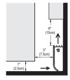
Between the front of the unit and objects located directly on the floor
