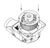
INSERT THE MOTOR ASSEMBLY IN THE CASING WHILE ALIGNING THE HOLES WITH THE SCREWS.
