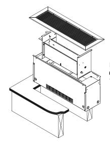
**FLOOR OPENING** 6 3/8" x (DIM. B + 1/4") 162mm x (DIM. B + 6.5mm)
