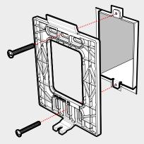
NOTE: Loosen the screw under the thermostat slightly to remove the mounting plate from the thermostat.
