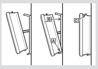
NOTE: If you need to remove the thermostat, follow step 1 in section 1, then use a straight screwdriver to unhook it from the top of the mounting plate.
