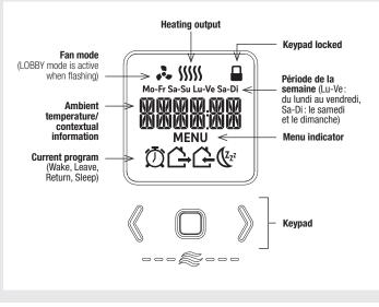
Operation mode: PROG / MANUAL (Programmable / Manual) When PROGRAMMABLE mode is selected, you can change the following settings:
