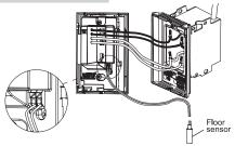
Reinstall the front part of the thermostat on the mounting base and tighten the screw at the bottom of the unit.
