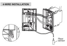
Reinstall the front part of the thermostat on the mounting base and tighten the screw at the bottom of the unit.
