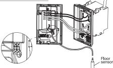
Reinstall the front part of the thermostat on the mounting base and tighten the screw at the bottom of the unit;
