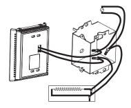
4. Using a screwdriver, loosen the screw retaining the mounting base and front part of the thermostat. Remove the front part of the thermostat from the mounting base by tilting it upward.
