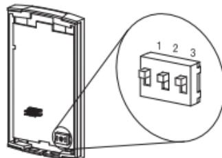
1. Early Start is used in Automatic mode only. When Early Start is enabled (on), the thermostat determines when to start heating so the Comfort temperature is attained at the start of periods 1 and 3. When Early Start is disabled (off), heating starts only at the start of periods 1 and 3; thus there is a delay before the Comfort temperature is reached.
