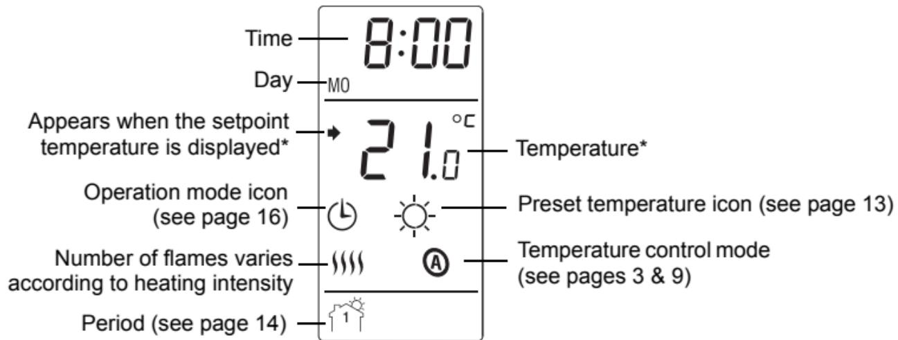
\* The thermostat normally displays the actual (measured) temperature. To view the setpoint temperature, briefly press either of the **▲▼** buttons. The setpoint will appear for 5 seconds. To change the setpoint temperature, press one of the **▲▼** buttons until the desired temperature is displayed. To scroll faster, press and hold the button.
