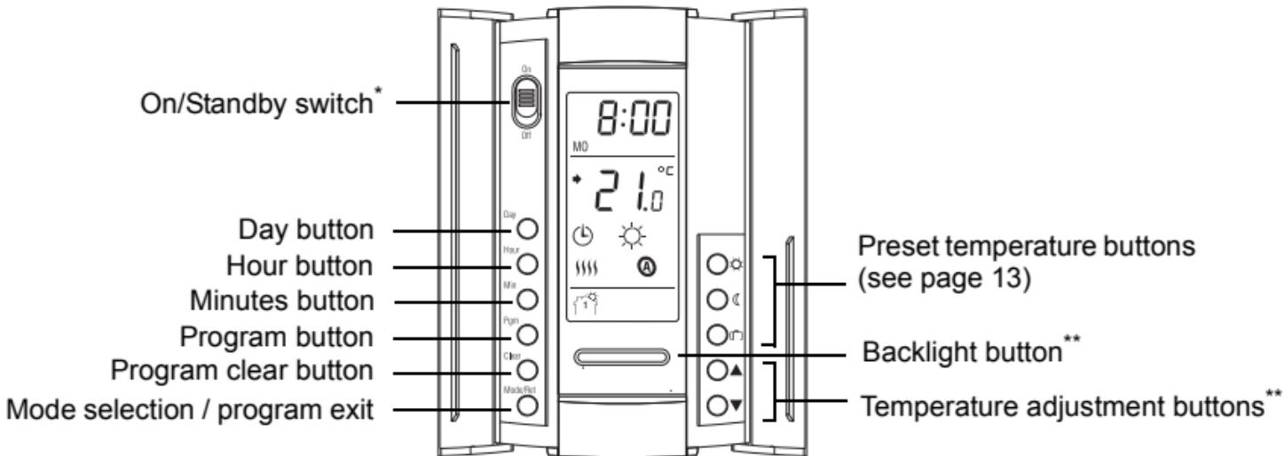
\* Place at Off/Standby to cut power to the heater (e.g., in the summer). This will not affect the time and temperature settings.
