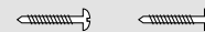
Two (2) No. 8 1 1/2 in. (38 mm) round-head screws to securely attach the fan heater mounting bracket.
